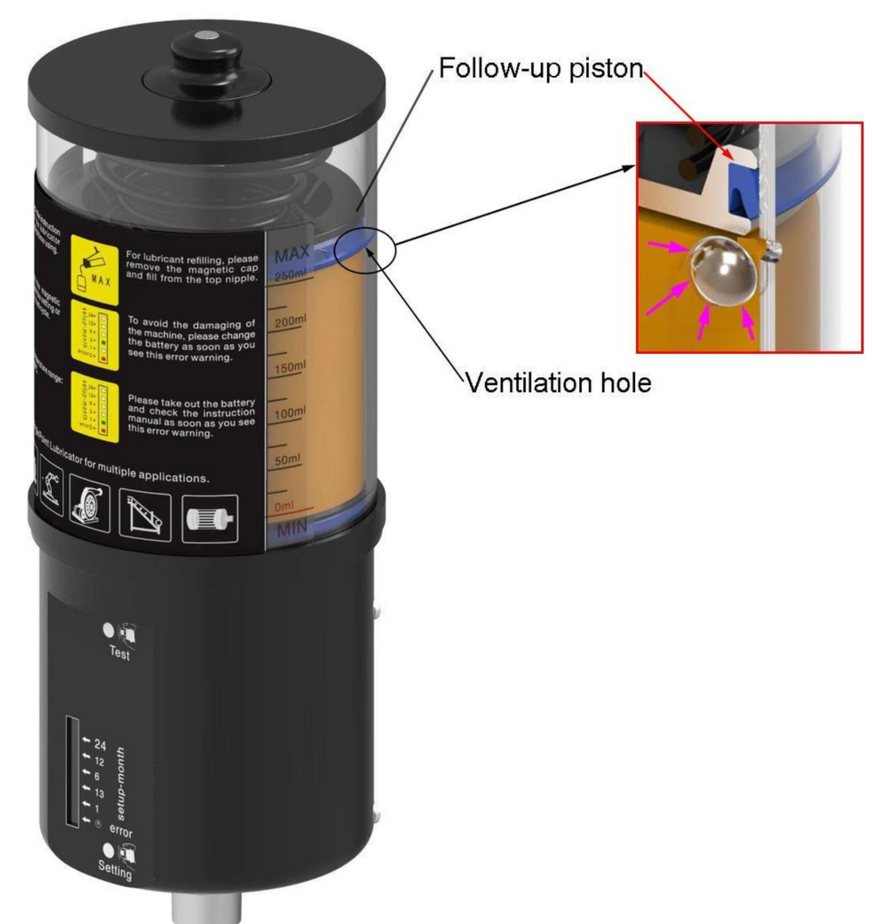
Fig. 7.2 Ventilation of reservoir
